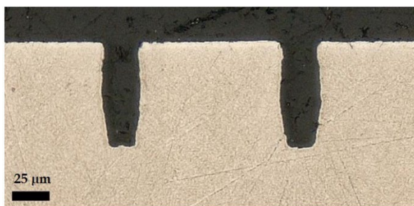
Cross-section view of 20 μm wide titanium trenches etched by SF 6 /O 2 /Ar plasma (2 μm/min). The Ni mask has been cleared before observation by optical microscopy.
